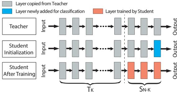
Figure 1: Transfer learning. A student model is initialized by copying the first  $N-1$  layers from a teacher model, with a new dense layer added for classification. The model is further trained by only updating the last  $N-K$  layers.
