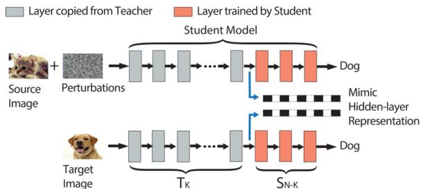
Figure 2: Illustration of our attack. Given images of a cat and a dog, attacker computes perturbations that mimic the internal representation of the dog image at layer  $K$ . If the calculations are perfect, the adversarial sample will be classified as dog, regardless of unknown layers in  $S_{N-K}$ .
